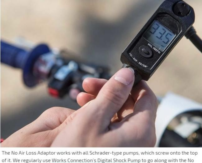
Once both pieces are secured to each other as well as the fork Schrader valve, the Digital Shock Pump screen displays the air pressure in the fork. You can add air by using the pump, or decrease pressure by pressing the micro-adjust air bleed button located just below the screen. With the air pressure below 100 psi, it measures in
